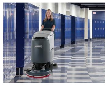
The extremely maneuverable SC500 features a low center of gravity and an easily accessible variable speed, pressure sensitive control paddle. That means virtually anyone can control the SC500's traction drive system, effortlessly propelling it forward at whatever speed feels comfortable and appropriate for the cleaning application.
