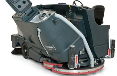
Tilt-out recovery tank makes inspection and clean-out much easier.
