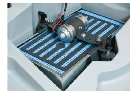
High-capacity Donaldson PowerCore® UltraWeb® nanofilter synthetic media filter with MERV 13 rating, combined with a variable-frequency shaker, offers high dust/dirt holding capacity in a more compact package, plus longer filter life and more consistent performance compared to conventional pleated filters.
