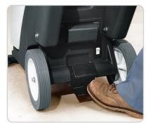
The base features an easy-to-use rugged on/off switch. A pedal for operating the front mounted tool assemblies is also included.
