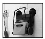
Handle folds down to reduce storage footprint; or machine can be hung on wall
