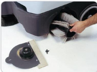
Main broom easily removed and replaced without the use of tools.
