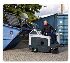
Hydraulic, high-dump hopper provides easy and safe disposal of large debris volume
