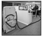
The VacRide can fit through doorways and standard elevators. An optional 25 foot hose and wand attachment lets you clean areas that the machine is unable to navigate.
