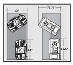
The Advance Adgressor® turns within a 63 inch (160 cm) aisle. This improves productivity by allowing the Advance Adgressor® to easily clean smaller aisles than the competition.
