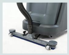
Front-mount squeegee is easy to install, and enables easy cleaning in both forward and backward directions. With a break-away design, the squeegee can be quickly engaged via the foot pedal.
