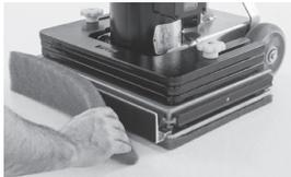
The FM810 XP comes with an innovative baseboard cleaner attachment as a standard feature. This simple device easily attaches to the front of the machine to provide a convenient alternative for cleaning baseboards without having to purchase a separate machine, or worse, getting down on your hands and knees to scrub.
