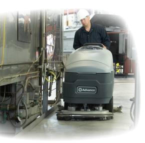
Walk-behind scrubbers are well suited to smaller facilities with a need for scrubbing and light debris pickup.
